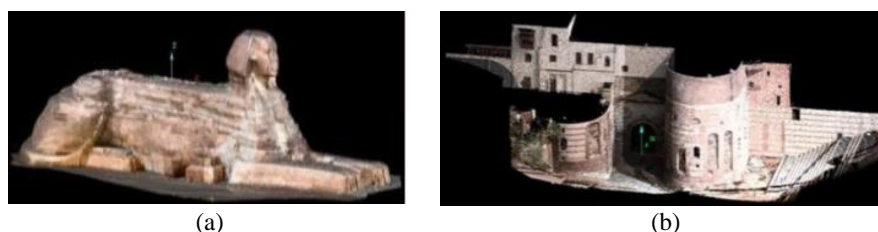
Fig.2 represent point cloud with vertex color that was obtained from the RIEGL LMS-Z620 laser scanner of (a) sphinx (b) Bawabet Amr
